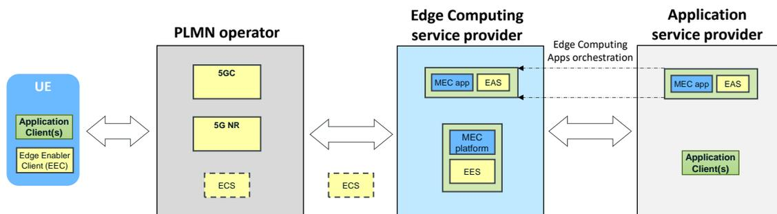
**Figure 5: Relationship of service providers in the edge computing network deployments**
