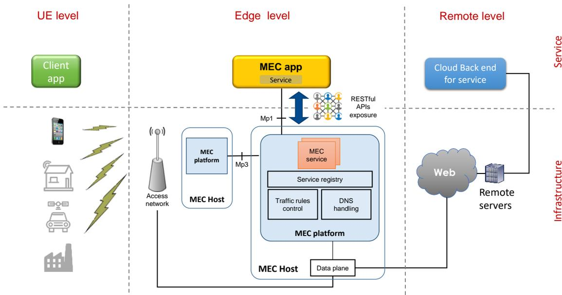
**Figure 2: MEC applications, interaction and service exposure**
