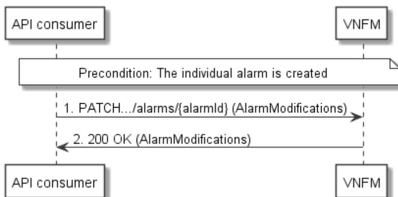
**Figure 7.3.3-1: Flow of acknowledging alarm**
