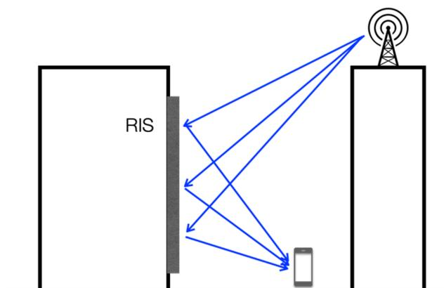
**Figure 5.1-4: BS serves UE in street canyon using large RIS on building walls**
