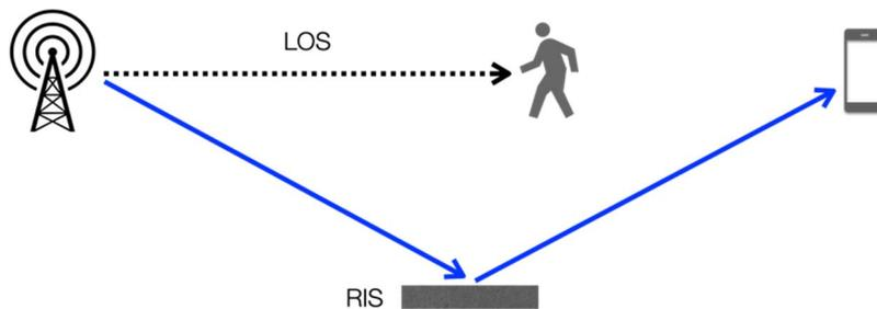
**Figure 5.1-1: RIS as a solution to blockage**
