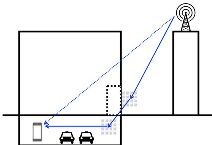
**Figure 5.1-5: RIS application in an O2I scenario, in which BS serves UE in underground garage using RIS**
