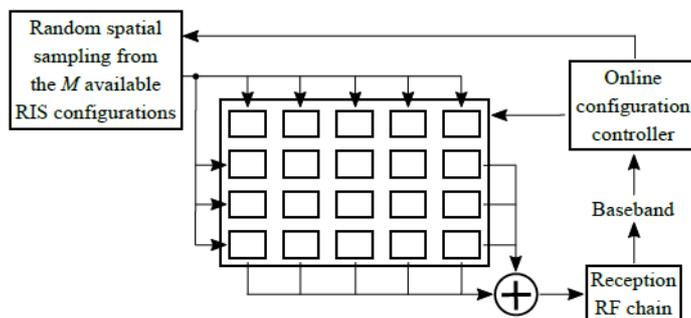
**Figure 4.3.6-1: Block diagram of a RIS hardware architecture including a single active reception RF chain, enabling the sensing of the impinging signal in baseband**
