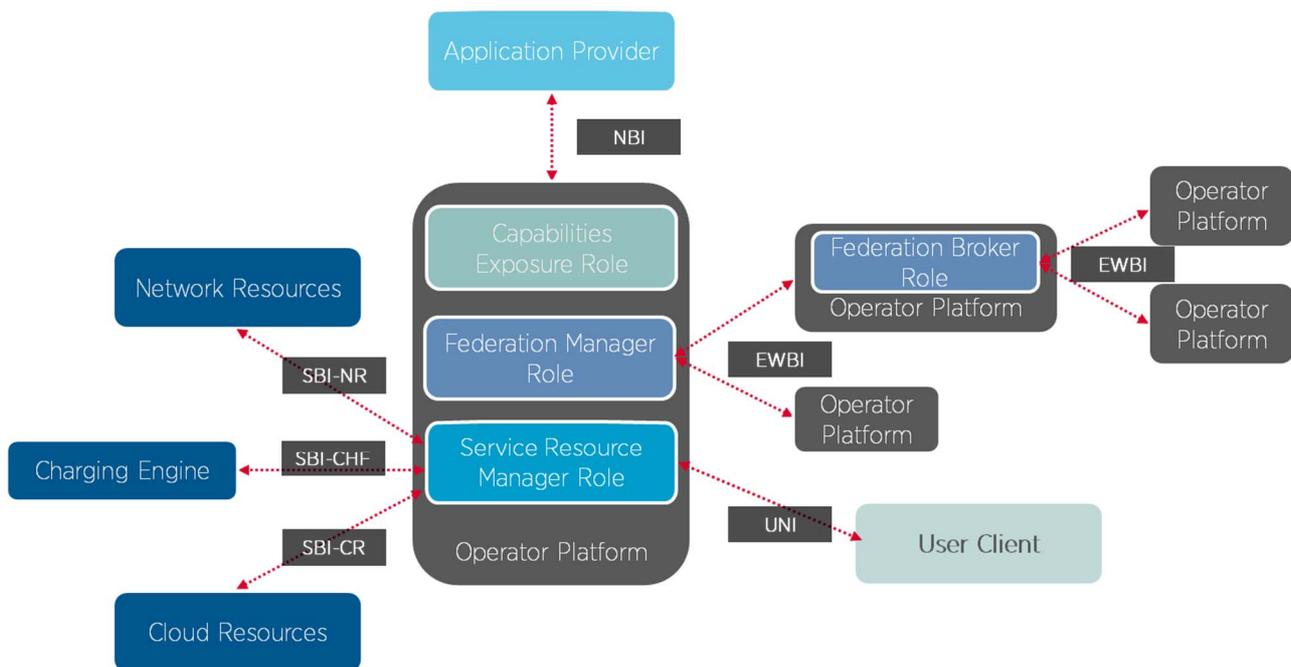
**Figure 4.2-1: High-level OP reference architecture (source: [i.1])**
