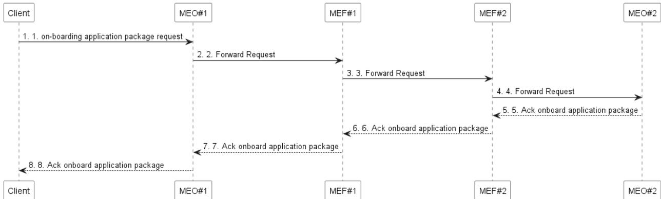
**Figure 5.2.2.5.2-1: On-boarding application package in MEC federation**
