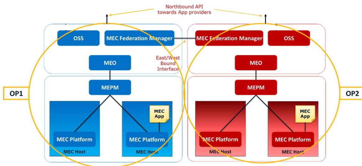
**Figure A-1: MEC federation and exemplary correspondence to GSMA OP interfaces NBI and E/WBI**
