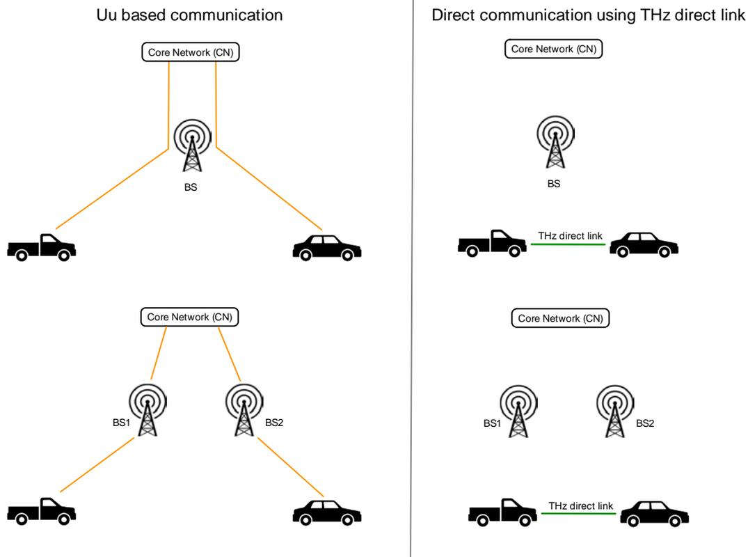
Figure 33: Offloading Uu communication (same BS or Different BS) to V2X direct communications
