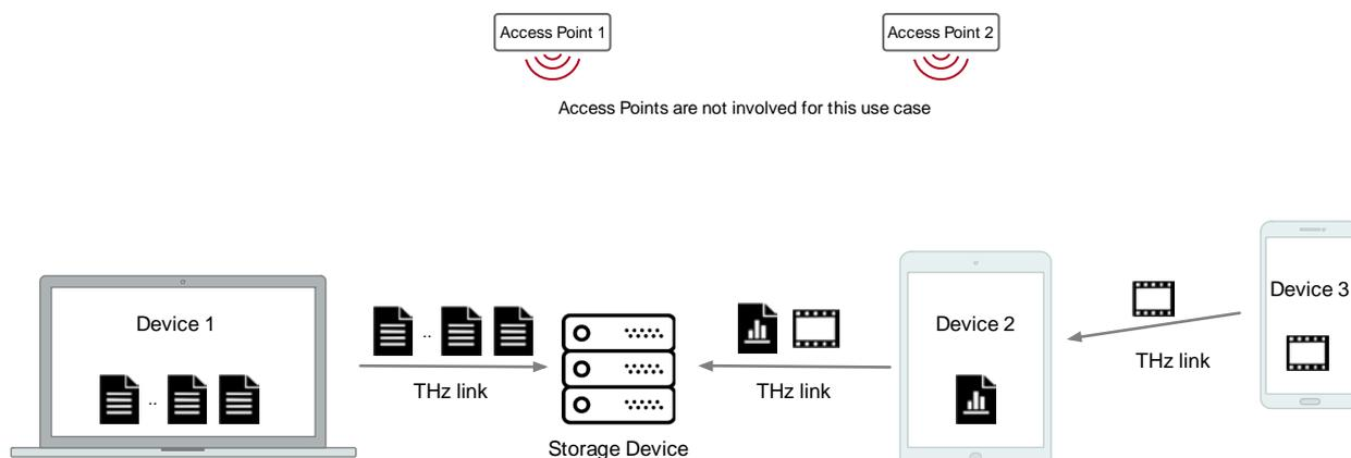
**Figure 29: High-speed wireless data backup**
