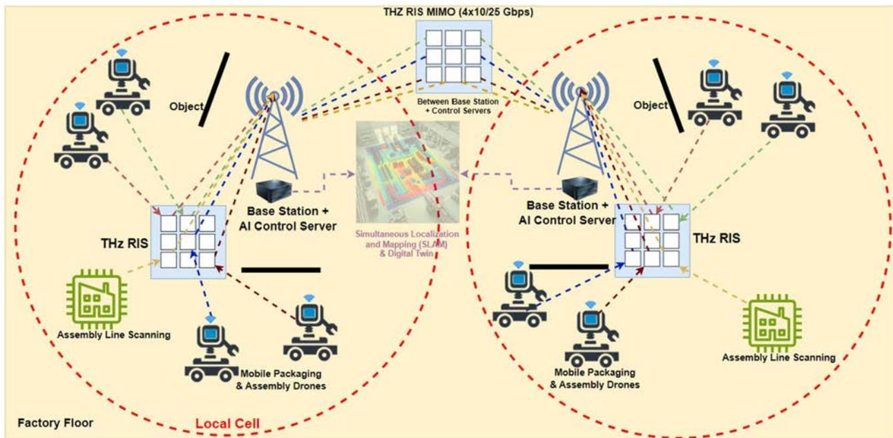
**Figure 6: Diagram showing robot to server communication utilizing a THz RIS and server-server connection between local cells using THz RIS multiple input multiple output communications**
