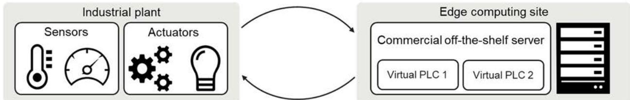
**Figure 19: Real-time industrial control at the edge**
