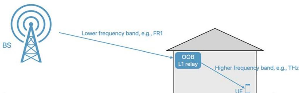
**Figure 26: OOB L1 relay assisted transmission for indoor user**
