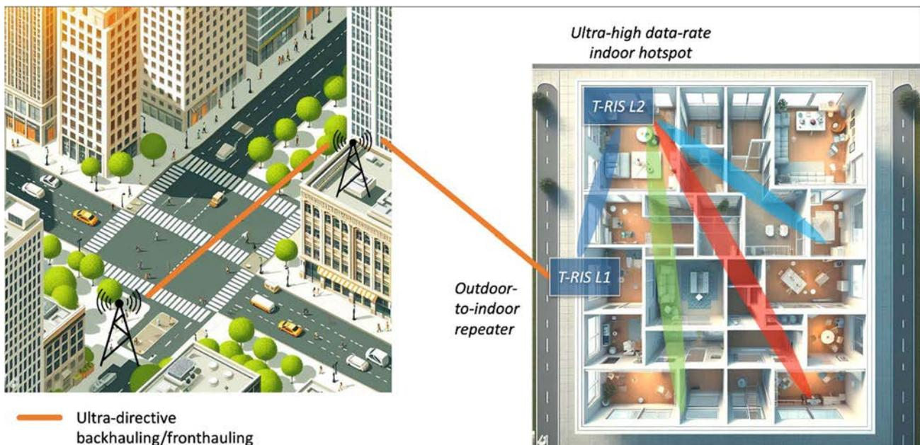
Figure 27: Use case on Ultra-high throughput for indoor users
