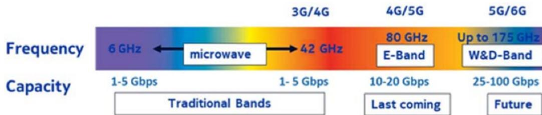
**Figure 13: Current bands allocation for fixed point to point radio links and their corresponding capacities**
