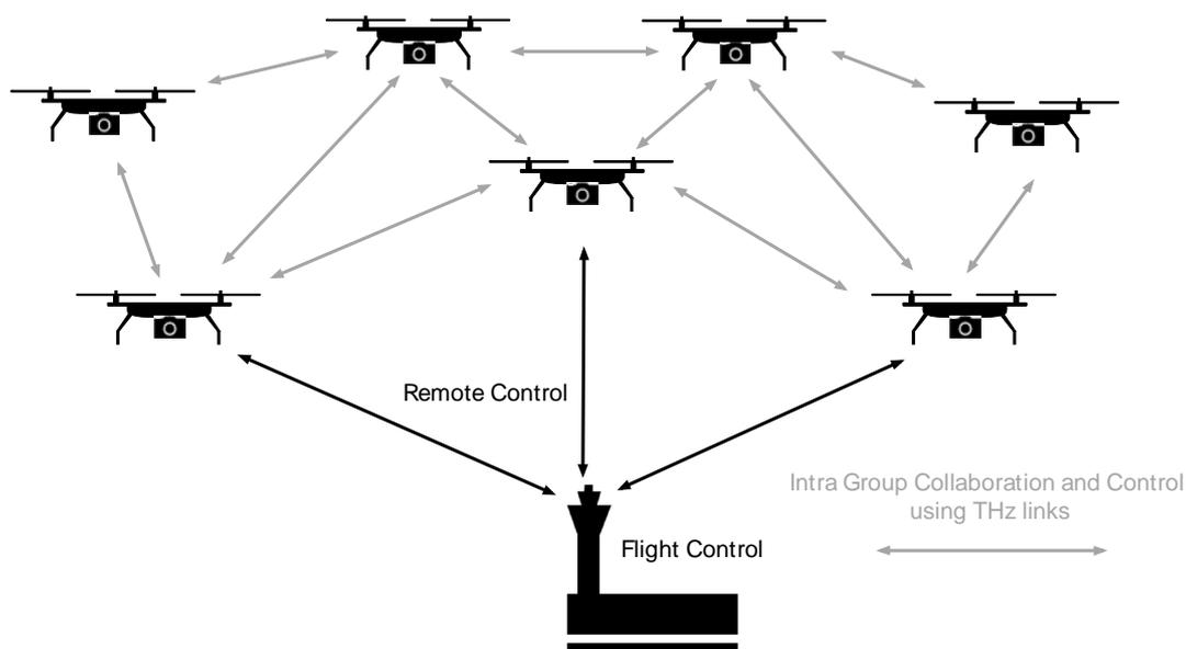
**Figure 5: Drone remote control and intra group collaboration**
