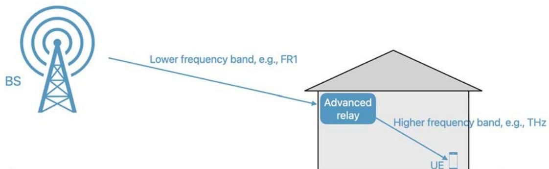
**Figure 37: Advanced relay assisted transmission for indoor user**
