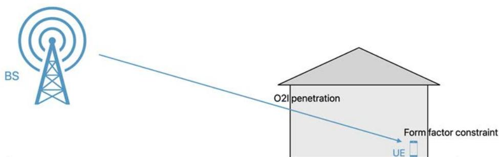
**Figure 23: Outdoor-to-indoor wireless communications for an indoor user**
