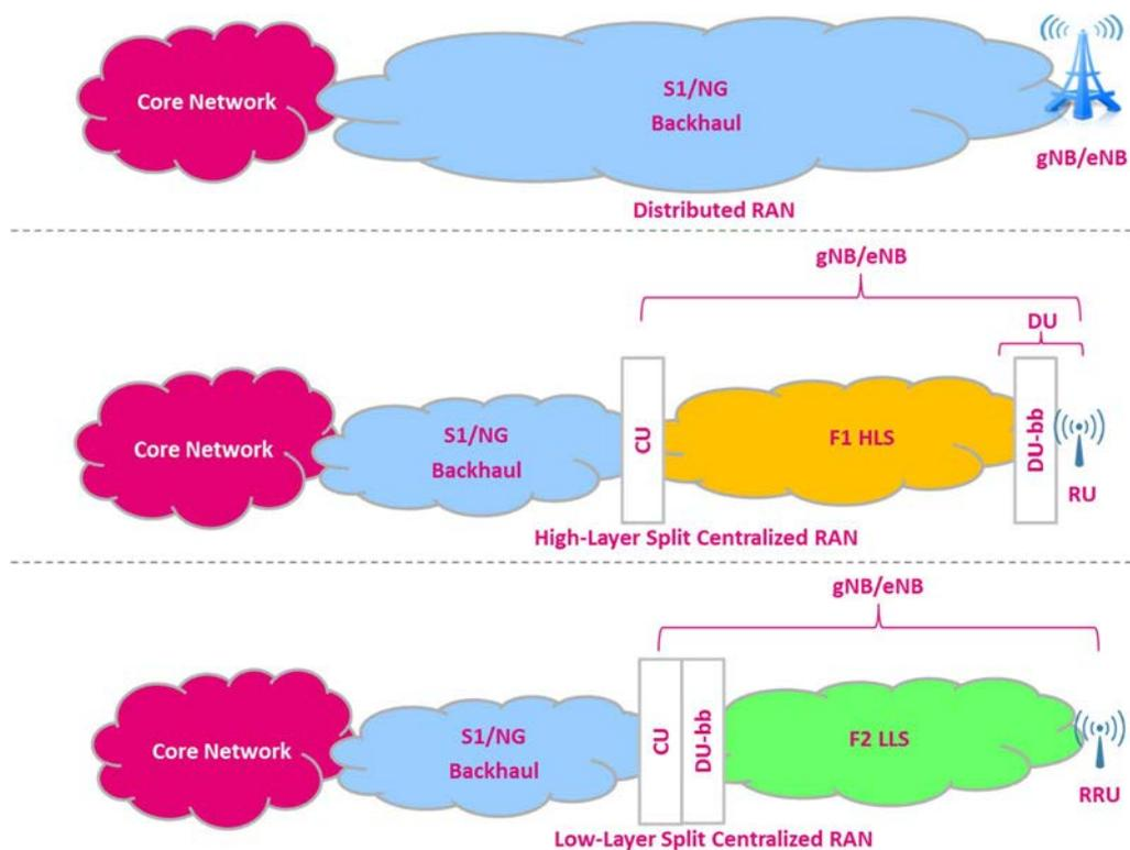
**Figure 12: Distributed and Centralized RAN Architectures**
