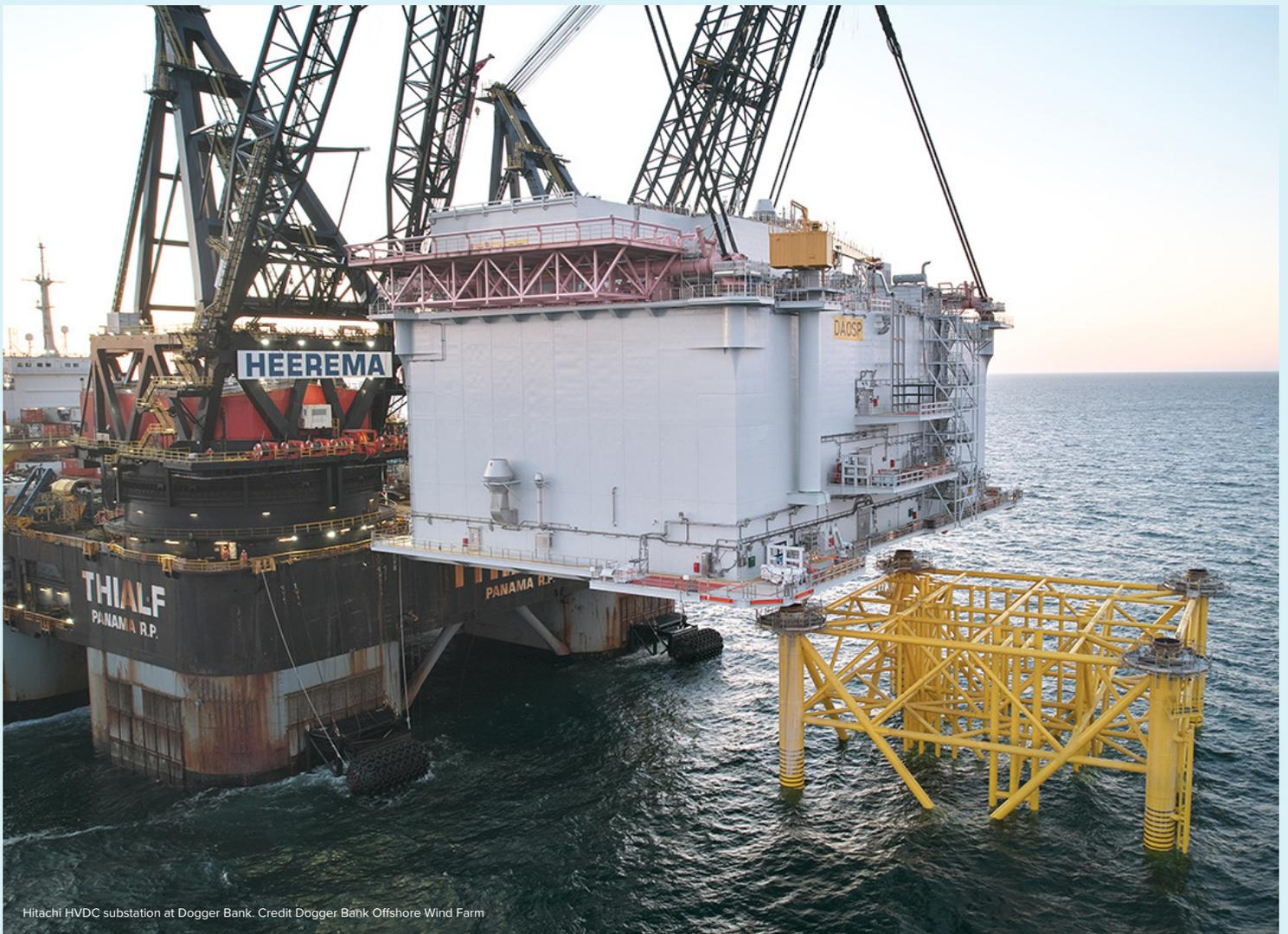
Hitachi HVDC substation at Dogger Bank. Credit Dogger Bank Offshore Wind Farm
